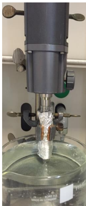
Figure 3 Mixing of hydrogel precursor with NFC fibers using an Ultra-Turax.
