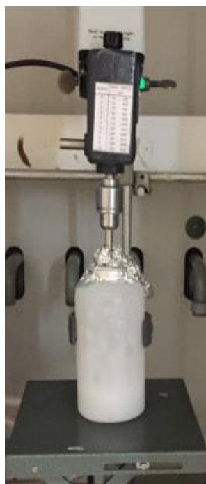
Figure 2 Mixing the NFC fiber for 20 min to homogenate the solution
