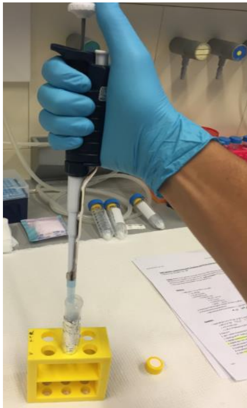
Figure 10 Resuspension of medECM polymers with NFC fibers using a pipette
