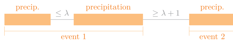
Figure B.1: Criteria for the event definition where one event can contain \lambda hours of precipitation free time, \lambda \in \{0, 1, 2\} .
