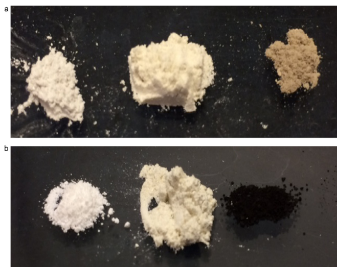
Fig. 9. (a) Powder samples of Ag(1%)-TiO 2 , Ag(3%)-TiO 2 and Ag(5%)-TiO 2 .
