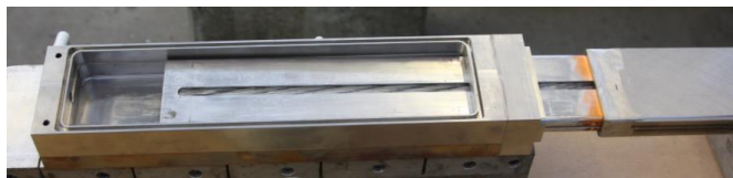
Fig. 5. The cable, in which the outer layer of Cu wires is replaced by two copper U-profiles, is being slid into the termination box.
