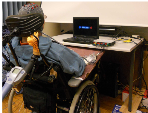
Fig. 2. Experimental setup showing the end-user, the EEG acquisition device and the computer screen showing the protocol feedback. In the experiment reported here, the horizontal cursor corresponding to the decoded MI task was replaced by the parachuting BCI game described in Figure 3.
