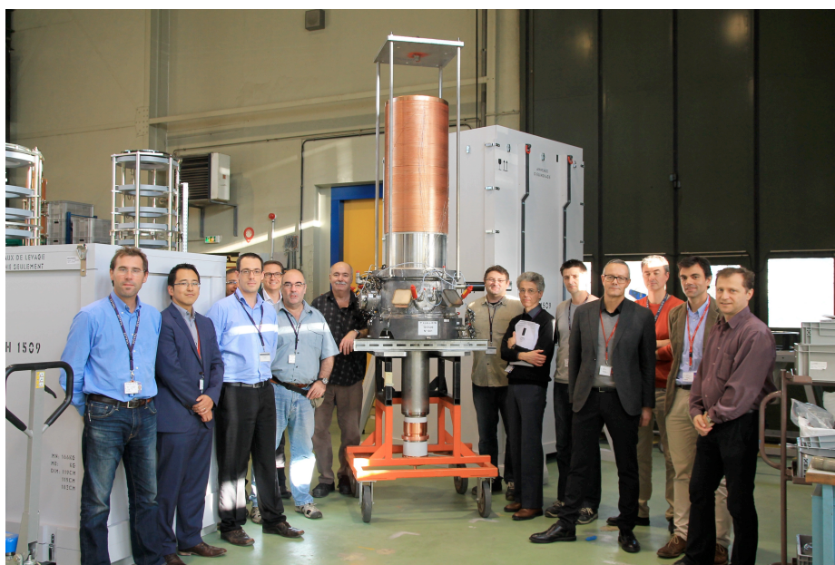
Fig. 2.5.1 CW gyrotron prototype during the factory acceptance test (FAT).
