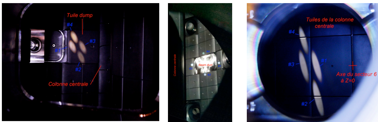
Fig. 2.1.4 Photographs of, pyrometer measurement locations at beam dump (white circles), beam entry (the 'duct') and the images on the central column.
