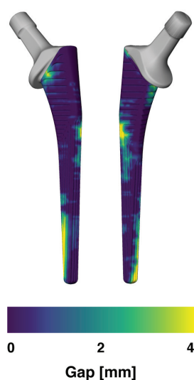
Figure A.1: Gap measured around the cementless femoral stem - Anterior/lateral and posterior/medial views of the stem displayed successively from left to right.
