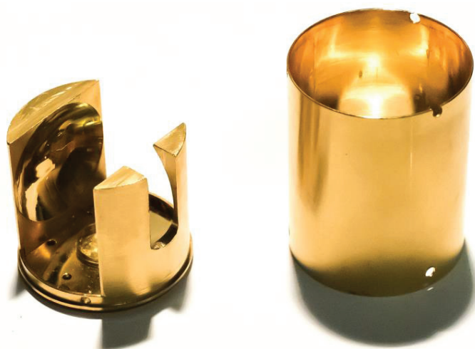
Fig. 4 Focusing structure of the microwaves in the cavity. Much of the space is occupied by the RF coils to optimize irradiation of the sample.
