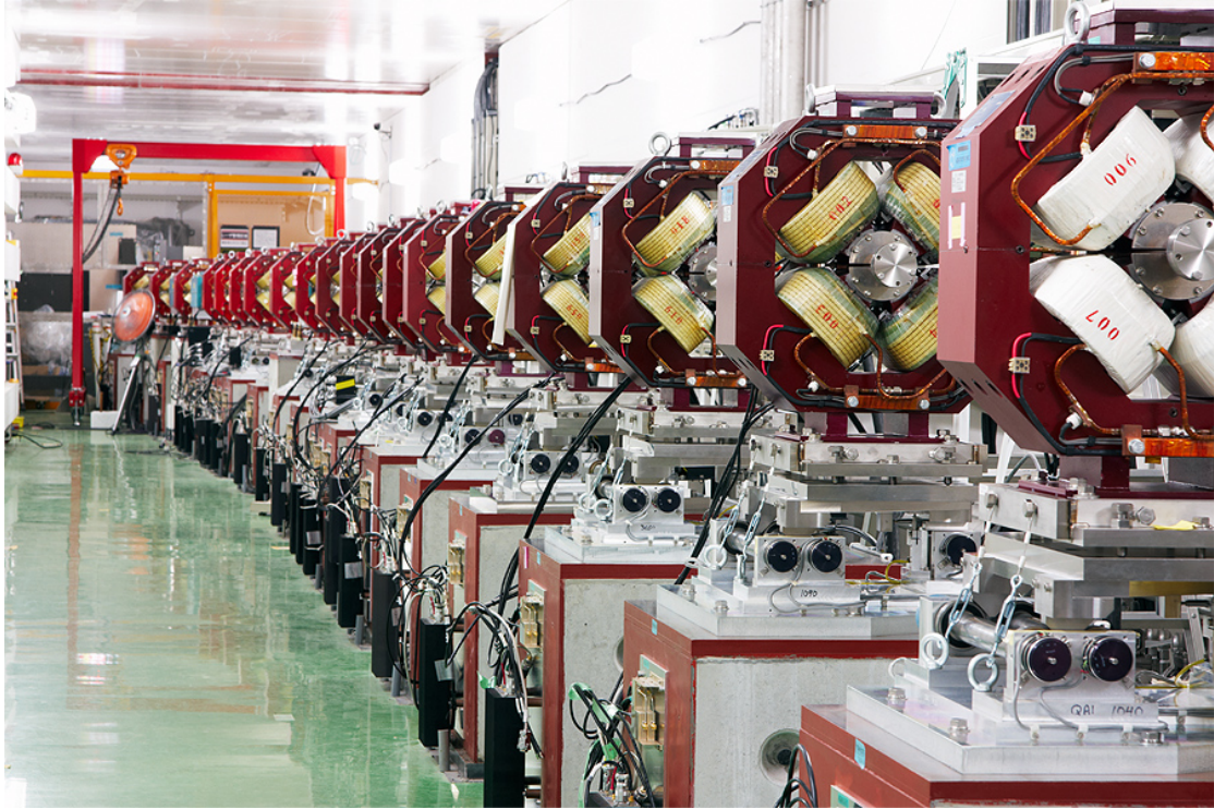
Figure 1.4 – A regular alignment of quadrupole magnets following the principle of strong focusing [KEK, Japan 2013].
