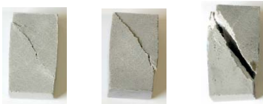
Fig. 4.42 Cracking behaviour in compressive strength test [20]
