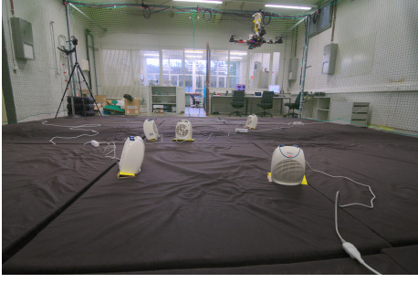
Fig. 4: Experiment in progress. Electrical heaters on the ground produce a surface temperature gradient to be estimated by the quadrotor.
