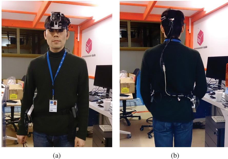
Figure 1.4 – The Personal Safety Device developed for the EDUSAFE project. (a) front: the compact camera and the Head-Mounted optical see through display are visible. The headset is also equipped with accelerometers and gyroscopes for more robust tracking. (b) back: a portable computing unit and a battery are fixed to the user’s belt. Images courtesy of m. Yuta Itoh.
