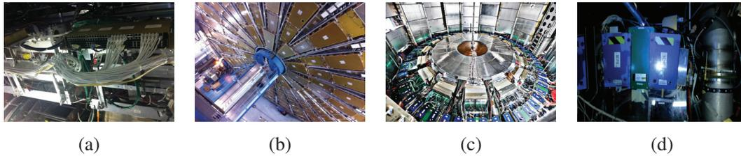
Figure 1.1 – Examples of the challenging visual conditions encountered in industrial environments: the ATLAS particle detector at CERN, Switzerland. Common sources of nuisance are (a) repetitive patterns, (b)-(d) drastic illumination changes (hand held torches are used for lighting dark places) (c) non-Lambertian surfaces.
