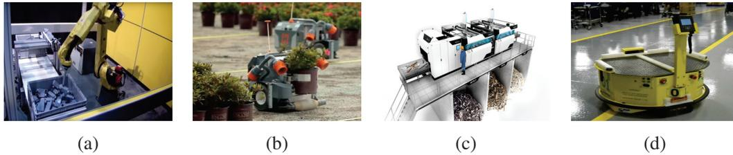
Figure 1.2 – Examples of industrial 3D tracking applications: (a) a robotic arm picking metallic pieces <sup>a</sup>; (b) a self-navigating robot displacing plant vases over a warehouse <sup>b</sup>; (c) an automated waste sorting system <sup>c</sup>; (d) an autonomous robot for goods transportation.<sup>d</sup>.
