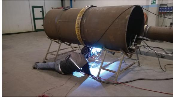
Figure 1.5 – The pipe welding machine in action during an indoor test. Guidance is provided by an expert, that closely monitors the welding torch while it turns around the pipe and manually adjusts the trajectory of the welding torch.
