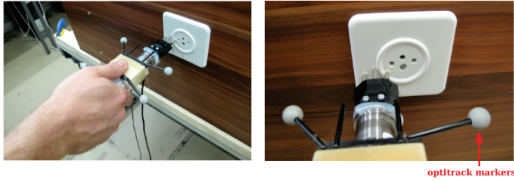
Figure 4.3: Human holding the cylinder plug holder, which is equipped with OptiTrack markers.
