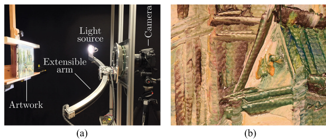
Fig. 20. (a) Photograph of our light dome for BRDF acquisition; (b) closeup of an artwork from which we captured the BRDF.
