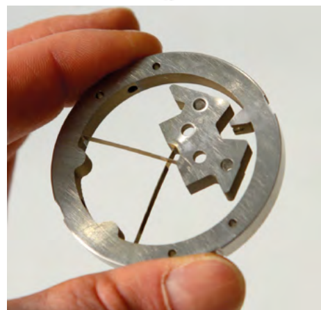
Fig. 2: (a) Classical pivot watch time base [12], (b) Flexure pivot watch time base demonstrator.
