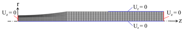
Fig. 3—Half of specimen modeled in Abaqus using an axisymmetric model together with the imposed mechanical boundary conditions.
