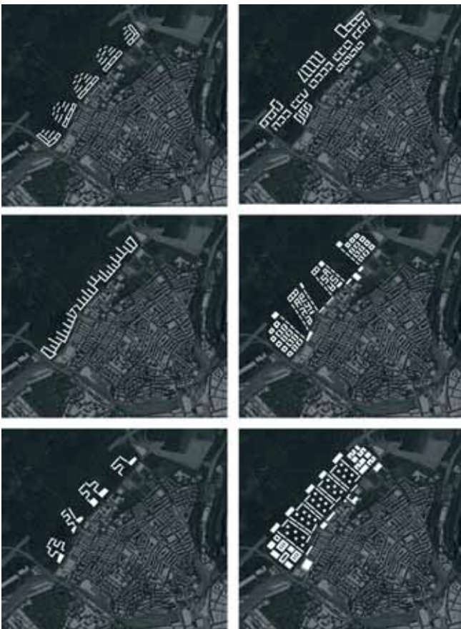
FIGURE 1: Exploring urban densification strategies under broader sustainability perspectives. Plans of the six visions developed for the Waldstadt site (from top to bottom): Transition , Interface , Outposts (left column), Checkerboard , Continuities and Hyperdensities (right column). Source: Rey (2013).
