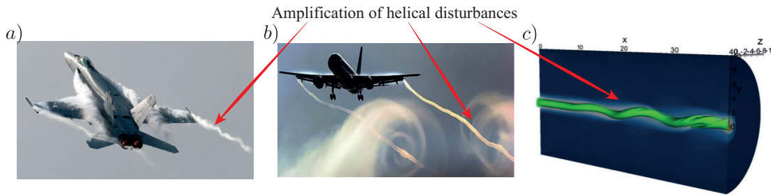
Figure 1.5: Spatial amplification of helical disturbances in trailing vortices in a) military or b) civil aircraft, and in c) the 3D numerical simulations of a Batchelor vortex harmonically forced (isocontour of axial vorticity, see text and chapter 2).
