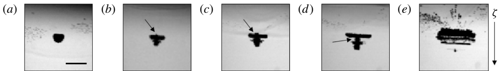
FIGURE 8. Selected images immediately after the collapse of bubbles near a free surface with (a) \gamma = 2.1 , (b) \gamma = 1.6 , (c) \gamma = 1.3 , (d) \gamma = 1.0 and (e) \gamma = 0.86 . Counter-jet formation is visible in (b), (c) and (d), indicated with arrows. The black bar shows the 1 mm scale. The arrow on the right shows the direction of \zeta .
