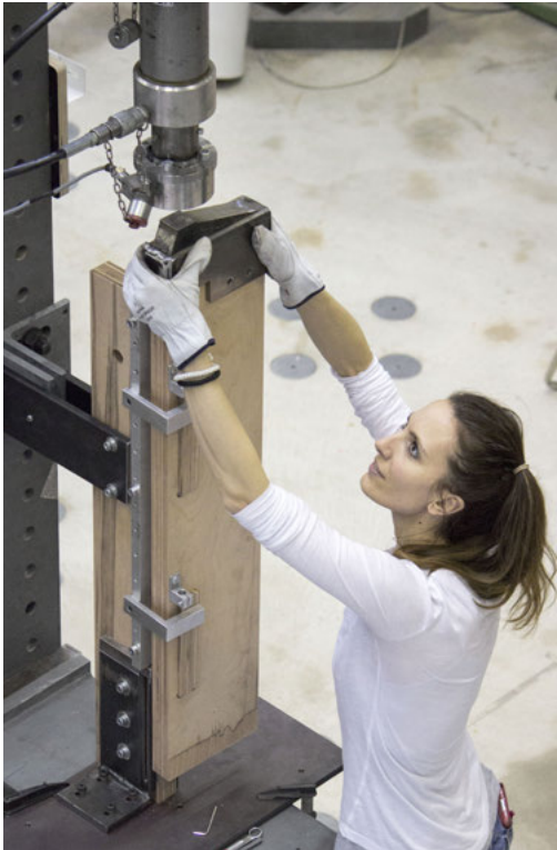
Figure 5. Experimental analysis of the influence of the tab rotation \theta_2 on the shear stiffness of the joints on 40mm cross-laminated LVL plates.
