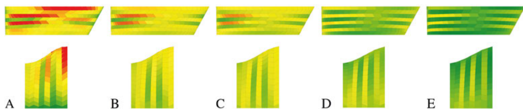
Figure 10. Balancing the fabrication requirements with the optimisation. From left to right different optimisation results are given by controlling the weights of constraints. First row is the top view and the second row is the side view of the last shell. Meshes are coloured according to a maximal angle \kappa between the edges of neighbouring faces. The comparison of \kappa angle, \alpha angle, and deviation from the target surface is given in Table 1.
