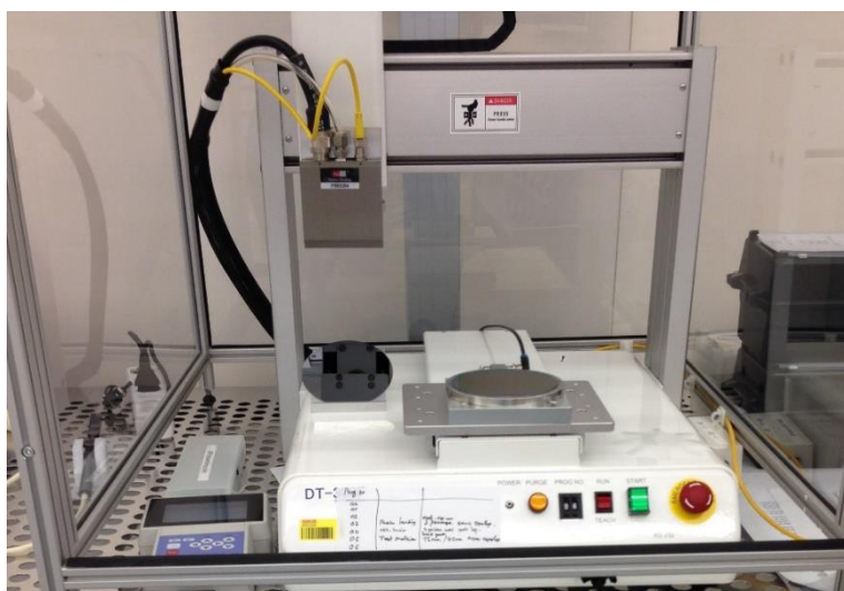
Figure 12: Surfex Atmosphere plasma used for surface activation (source: CMi website)
