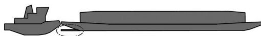
Figure 1. Sketch of pusher tug (left) and barge (right), with wave-reducing flap at barge stern.
