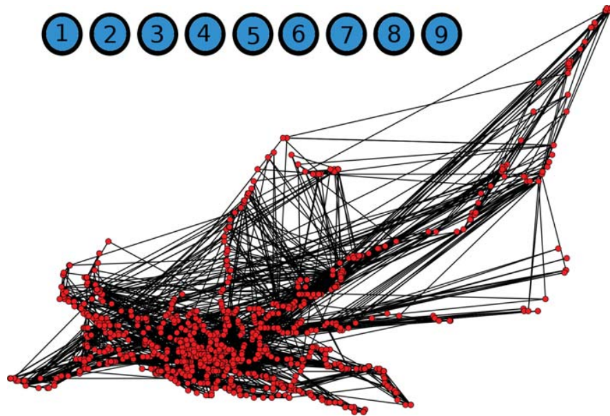
Figure 16.1 – The generated network for Lausanne’s street segments for LDSA estimation model. Each red node represents the center of one segment while the black lines between two nodes represent the correlation between the LDSA values of two segments. The big 9 blue nodes represent the nine explanatory variables which are in fact connected to all other nodes. For increasing the readability of this figure, we have removed all the edges between the blue nodes and the red nodes.
