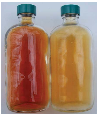
Figure 1.1 – Nitrogen dioxide ( \text{NO}_2 ) has a reddish-brown color. The intensity of the color varies with temperature, as \text{NO}_2 converts to the colorless gas dinitrogen tetroxide ( \text{N}_2\text{O}_4 ) at low temperatures, and converts back to \text{NO}_2 at higher temperatures. The bottles in this photograph contain equal amounts of an \text{NO}_2/\text{N}_2\text{O}_4 mixture at different temperatures. (Image source: Public Domain)
