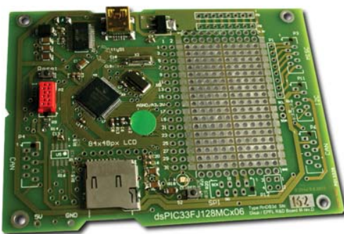
Figure 6.1 – The DISAL R&D Board - a flexible fast prototyping and development electronic board built around a dsPIC33F micro-controller.
