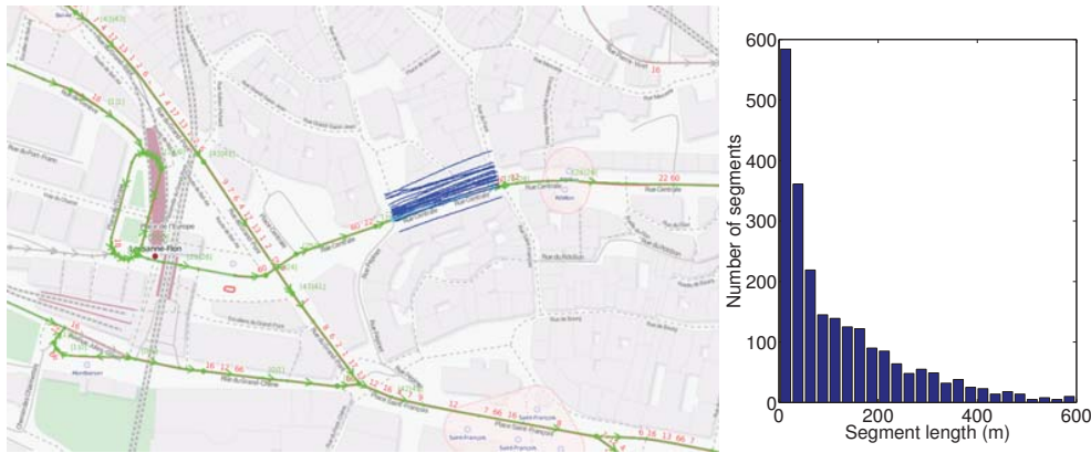
Figure 15.1 – Left: One snapshot of the developed street matching software. In this example the blue lines show the reported trajectory traces of the buses during one week in one segment. Due to localization errors, the blue traces are deviated from the actual position of the street segment. Our street matching algorithm has matched all of them to one segment. The green lines show the other segments that buses have passed during this period. Right: The histogram of length of the street segments. Most of our segments are shorter than 25 meters.
