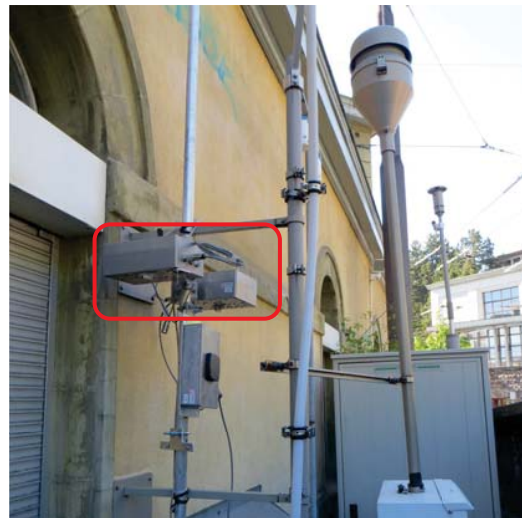
Figure 7.3 – A sensor node equipped with two gas sampler boxes deployed in parallel at the Lausanne NABEL station.
