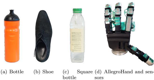
Figure 17: (abc) Exp 4 : Models of the grasped objects by the real robot. (d) The AllegroHand with fingers covered with Tekscan tactile sensors. Each patch is a matrix of 4 \times 3 or 4 \times 4 taxels ( 4 \times 15 for the base of the index finger)
