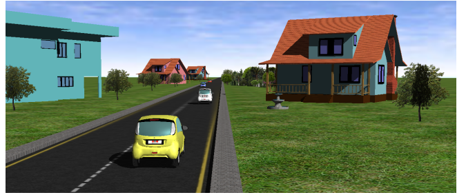
Fig. 4. Setup in the Webots simulator. The ego car (yellow) drives on a straight road behind the cooperative car (white), while two non-cooperative cars drive in the opposite direction.
