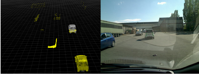
Fig. 2. Experimental setup. Left: ego vehicle (yellow), cooperative vehicle (white), and lidar point cloud of the surrounding of the ego vehicle (legacy vehicles are easily identifiable). Right: View from the web camera installed behind the windshield of the ego vehicle.
