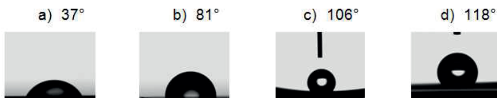
Figure 5.4b. Restoration of the initial hydrophilicity on the PE-TiO 2 as a function of times in the dark: a) 6 h, b) 12 h, c) 18 h and d) 24 h.
