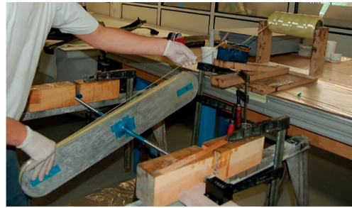
Figure C.3. Application of aramid fibers around mold (left), progression of specimen (right).
