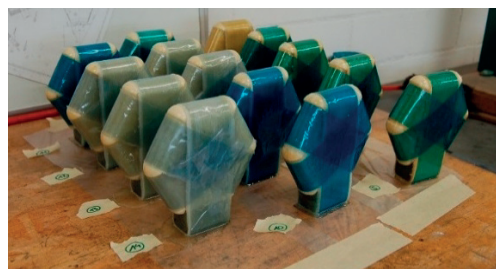
Figure E.4. Curing of GFRP and AFRP specimens.
