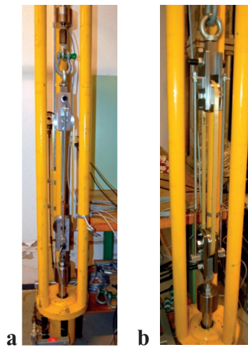
Figure C.10. Set-up for creep experiment.
