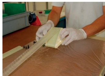
Figure E.3. Wrapping of foam specimen, inner layer (left), intermediate layer (right).
