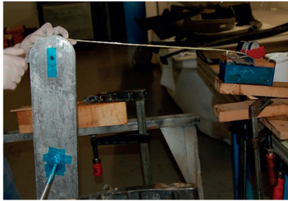
Figure C.3. Application of aramid fibers around mold (left), progression of specimen (right).
