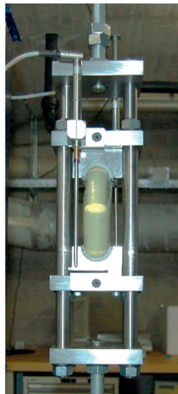
Figure 3.11. A/GFRP hexagon sandwich: creep experiment, set-up S1.
