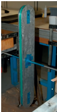
Figure C.4. Application of blue tape for plane section.
