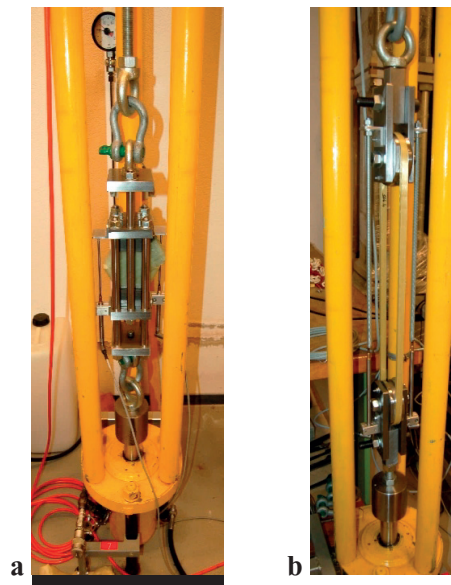
Figure 5.4. Creep set-up of a) GFRP hexagon sandwich component and b) AFRP loop component.
