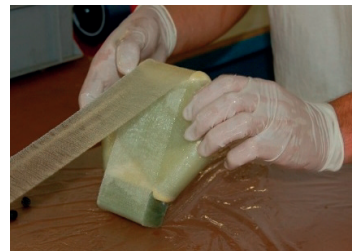
Figure E.3. Wrapping of foam specimen, inner layer (left), intermediate layer (right).
