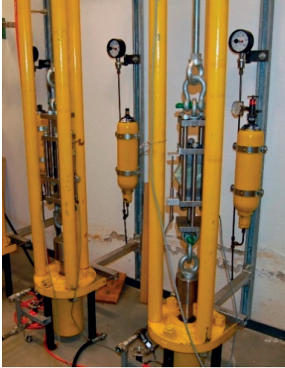
Figure E.7. Set-up for compression creep experiment.
