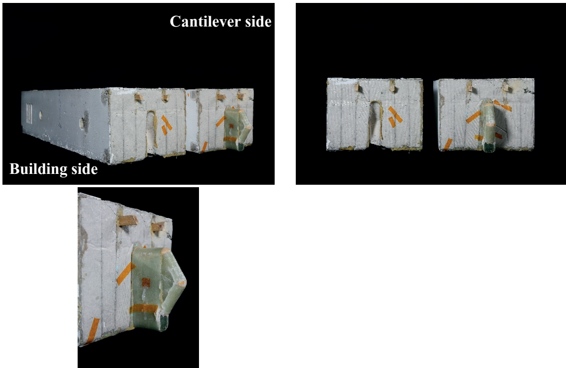
Figure G.11. Beam G400-1, F_u=25.8 kN.
