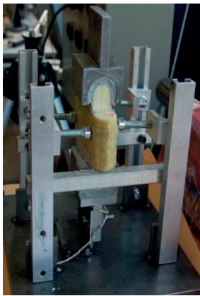
Figure B.5. Application of adhesive layer.
