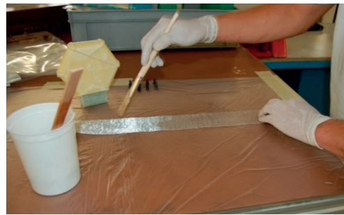
Figure E.2. Application of resin to fabric.
