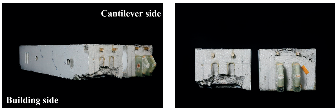
Figure G.9. Beam G400, F_u=40.7 kN.
