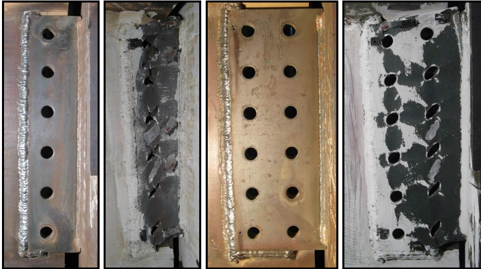
Figure 9: Photographs of post-test deformations for welded connections “L” shape weld (Test Configurations 6 & 8)
