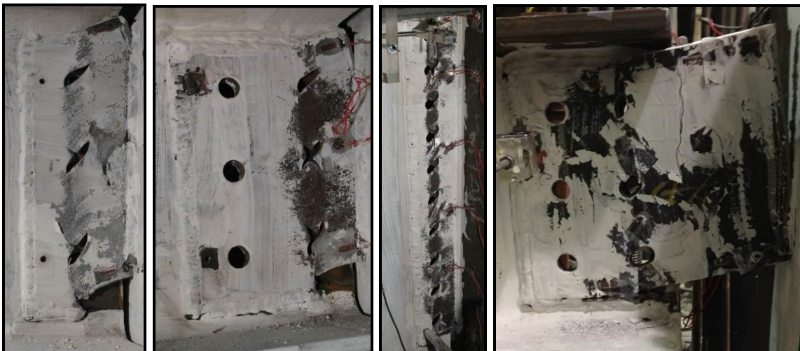
Figure 8: Photographs of post-test deformations for welded connections "Partial C" weld (Test Configurations 2,4,9 & 11)
