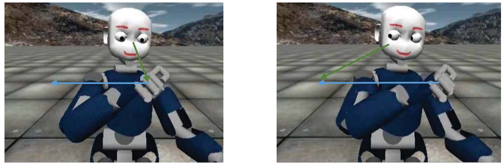
Figure 1. The iCub robot (in simulator) acting as the leader in the mirror game, generating random sinusoidal trajectories. (Left) the gaze is fixated on the hand. (Right) the gaze precede the hand. The blue arrows shows the next hand movement and the green arrows show the current gaze fixation point.
