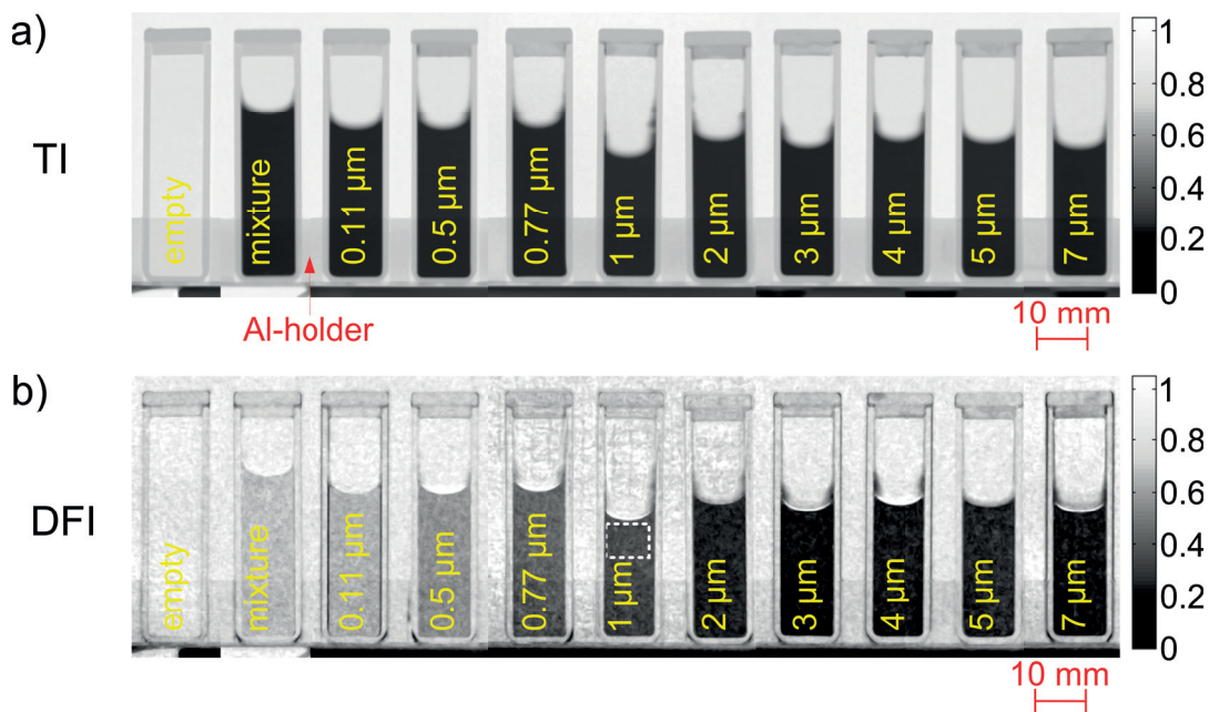
Figure 3.9: a) TI showing an empty quartz glass cuvette, a cuvette filled with the D_2O/H_2O homogeneous mixture, and cuvettes with particle solutions with varying diameter from 0.11 \mu\text{m} up to 7 \mu\text{m} . No obvious contrast difference between the different particle size solutions is obtained in TI. b) DFI of the same cuvettes as in the TI above. In contrast to the TI results the DFI shows clear differences for varying particle sizes. In both images the aluminum holder is slightly visible in the lower part.
