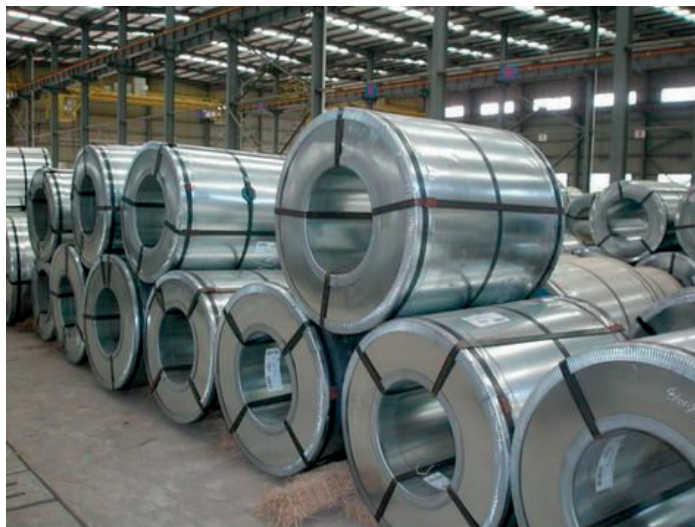
Figure 1.1: Coiled electrical steel sheet, as they are produced in industry. The sheet itself has a thickness of 350\ \mu\text{m} and the roll is about 1.5 m in diameter [1].
