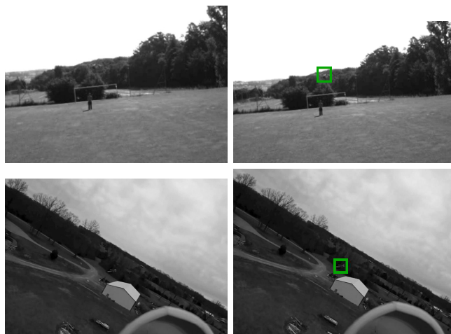
Figure 1: Detecting a small flying object against a complex moving background. (Left) It is almost invisible to the human eye and hard to detect from a single image. (Right) Yet, our algorithm can find it by using appearance and motion cues.
