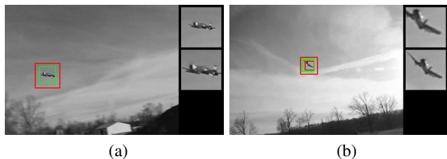
Figure 19: Scale adjustment. The red bounding box shows the original detection and the green one the position adjusted for scale and motion. The thumbnails on the right are zoomed-in versions of the detections, with the top one illustrating the original detection and the bottom one showing the one after being motion and scale are adjusted. (best seen in color)
