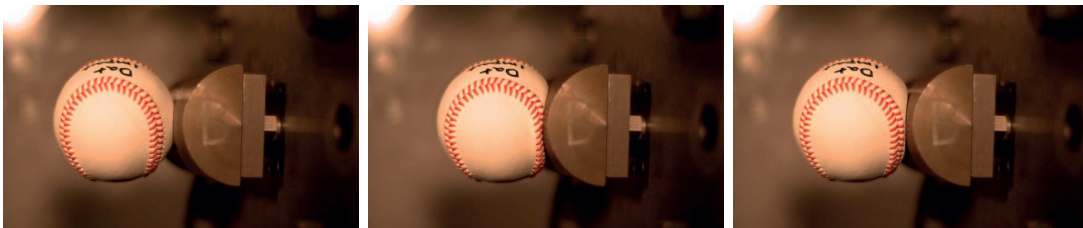
Figure 1.3: An impact of a baseball colliding with a rigid cylinder serving as a bat was captured using a very high speed camera. Video-based 3-D modeling of ball deformations could help improving simulation results and designing protective equipments.
