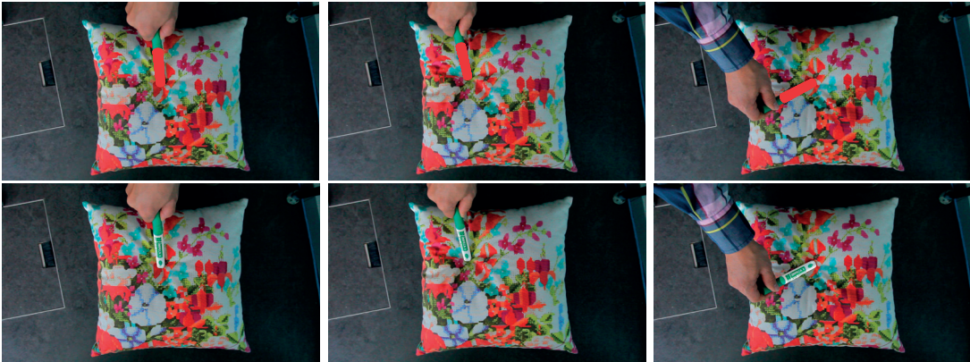
Figure 5.13: Results of tracking the 3-D pose of a small pen using direct image alignment and render-based template generation. Top row: Reprojection of the pen 3-D model on the input image (in red). Bottom row: Template generation for the next frame by rendering the 3-D model on the current view.
