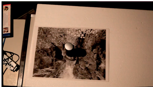
(a) The casted shadow indicates the lighting direction. The world coordinate system coincides with the camera coordinate system
