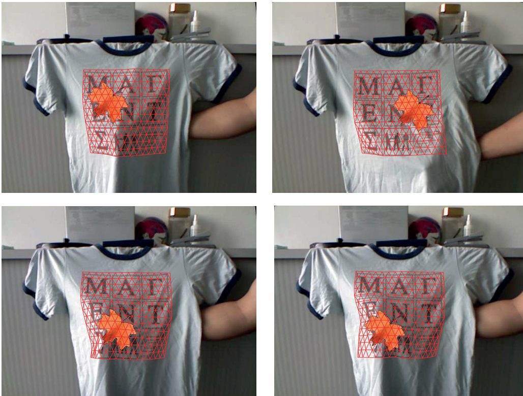
Figure 4.18: Our representative reconstructions on the t-shirt dataset with artificial occlusions added. Bottom right: a tracking failure case when occlusions appear at areas with large deformations.
