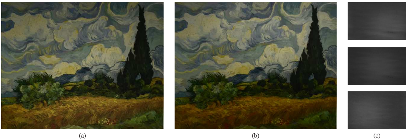
Fig. 18: We acquired a replica of Van Gogh’s ‘Wheat Field with Cypresses’, using our hand held acquisition strategy. Image plane has a resolution of 427 \times 544 . Illumination plane has a resolution of 75 \times 49 . (a),(b) shows relighted images for three different light positions. (c) shows some randomly selected largely diffuse LTFs.
