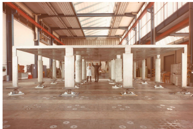
Figure 1.3 Reduced-scale punching test on a continuous slab by Ladner et al. [Lad77], supported on 16 columns and loaded uniformly on the top surface (picture courtesy to Mr. Heini Lippuner and Dr. Marc Ladner)
