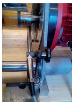
(a) Infrared sensor
