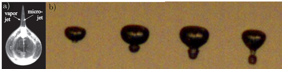
Figure 4. (a) Gravity-induced jetting, directed upwards, from [9]. (b) Downwards jetting observed during the collapse of a beer bubble under the reverse acceleration due to the vertical impact. The time step between images is 24 \mu\text{s} .
