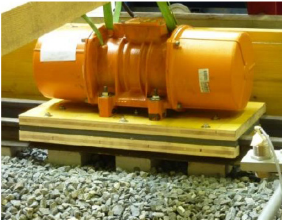
Figure 14: Physical model modified for the tests with vibrations
