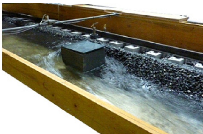
Figure 10: View of the flow around the manhole with an upstream backwater curve
