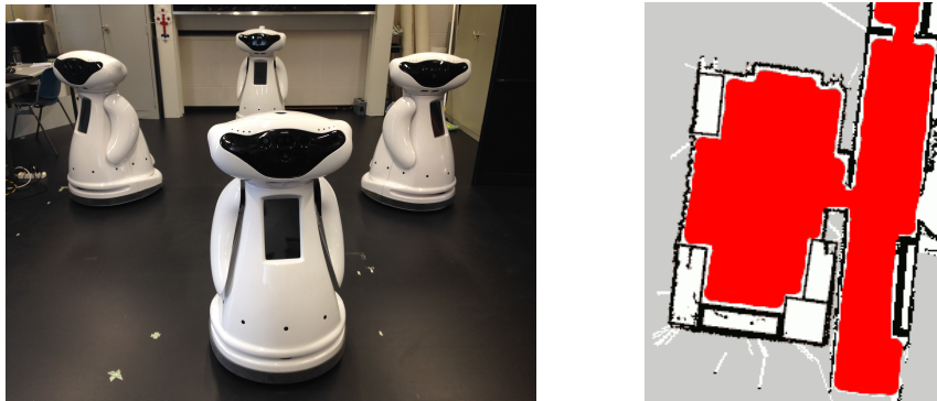
Fig. 1: Left: The Mbot robots. Right: Map of the environment with area allowed for navigation marked in red.
