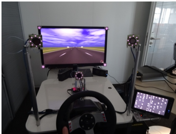
(a) The three-camera acquisition setup
