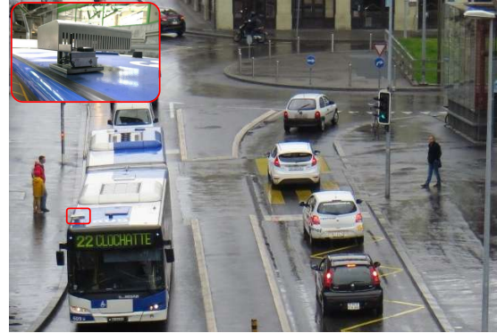
Figure 3. One of our sensor nodes anchored to the roof of a Lausanne bus. The gas sampling system used in this paper is a sub-module of this real-world platform.
