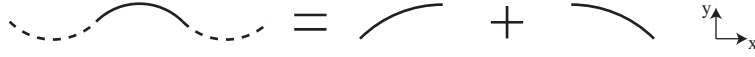
Figure 3.7: Additional symmetries of buckled beams: the half period possesses a reflection in the y direction also.
