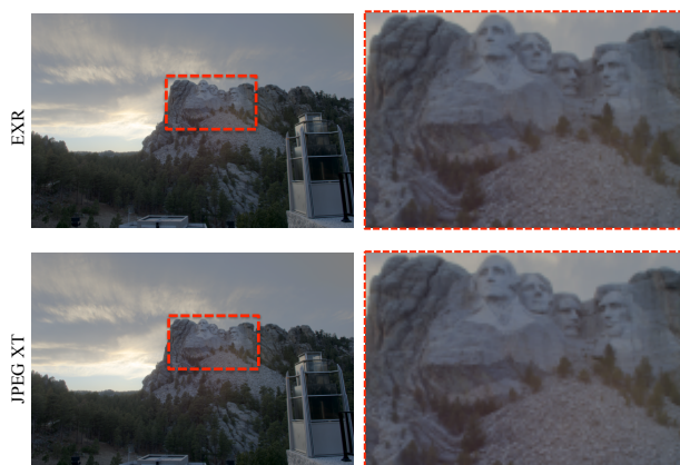
Fig. 1 Original (EXR) and compressed and decoded image (JPEG XT), both tonemapped and scaled for the purpose of printing. The original image size in the OpenEXR (PIZ compression) format is 39,4 MB (24.0 bpp) large, the compressed size is 3,4 MB (2.0 bpp), less than one tenth of the original file size.
