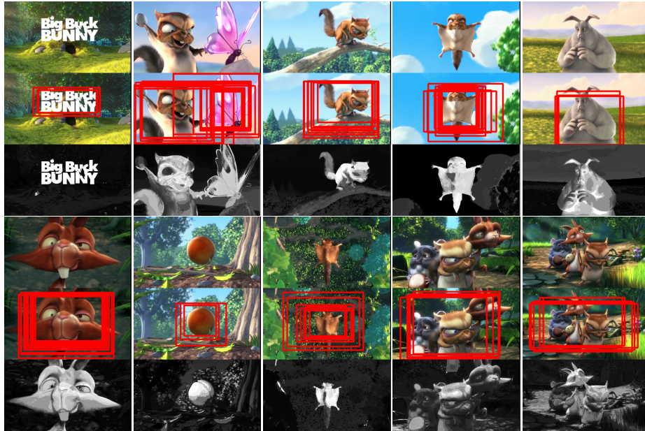
Fig. 8. 10 frames from the video “Big Buck Bunny”. The first row shows the original frame, the second row position and the size of the most salient objects, and the third row the saliency map of the frame.
