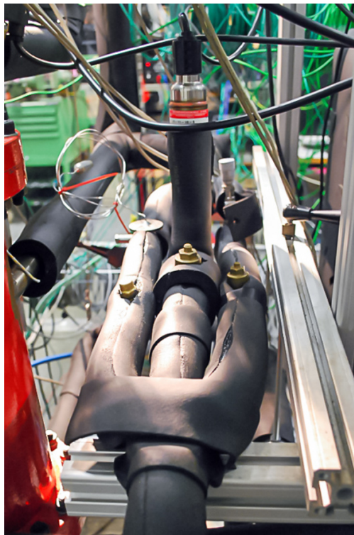
Figure B.1: BWP expansion devices section
