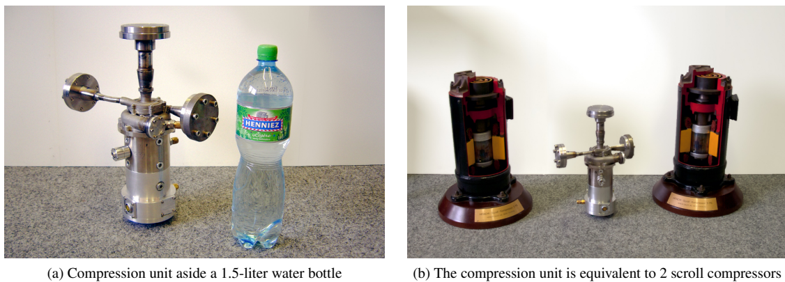
Figure 2.2: The volume and the weight of the twin-stage compression unit are several times lower than a single-stage scroll compressor. The 6 kW twin-stage compression unit is roughly equivalent to 2 single-stage 3 kW scroll compressors.
