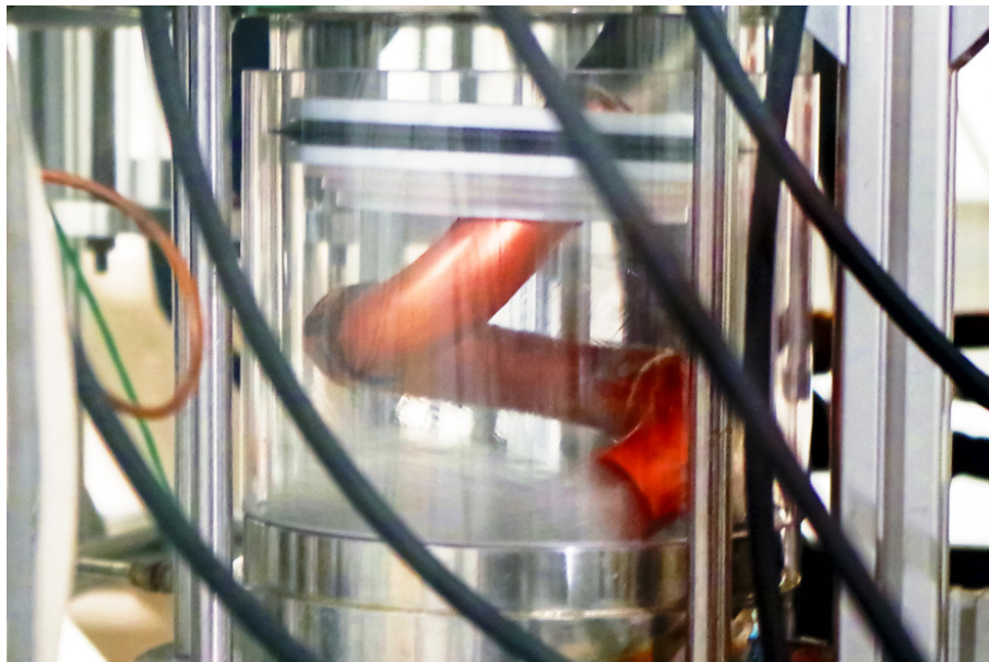
(b) Version #5 (big central hole, with a seal and shapes to send the liquid back down the economizer on the sides)
