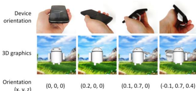
Figure 6. Dependence of the device orientation and the rendered 3D graphics.
