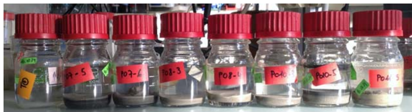
Figure 23 – The organohalide-respiring bacteria (OHRB) enrichment culture microcosms from aquifer sediments after 130 days.
