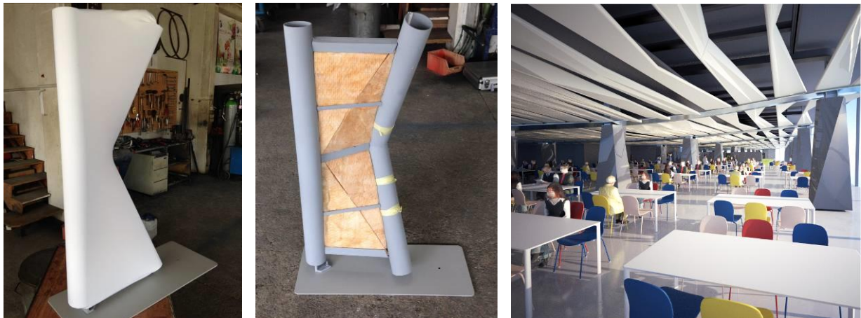
Figure 3: Sail prototype covered with fabric (left); Sail prototype without fabric (centre); photorealistic view of the restaurant (right).
