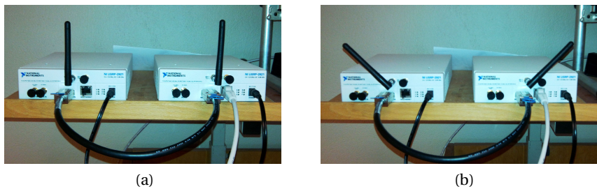
Figure 5.14: Polarization of the receive antennas; (a) vertically polarized, (b) perpendicular angled at 45^\circ .
