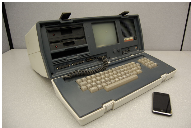
Figure 1.1 – Evolution of microelectronic technology: An Osborne Executive portable computer, from 1982 with a Zilog Z80 4MHz CPU, and a 2007 Apple iPhone with a 412MHz ARM11 CPU; the Executive weighs 100 times as much, has nearly 500 times as much volume, cost approximately 10 times as much (adjusted for inflation), and has about 1/100th the clock frequency of the smart-phone. [source wikipedia]
