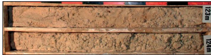
Figure 3.6 Drill core photo, example of non-cohesive fault rock (kakirite), after Fasching and Vanek, (2011).
