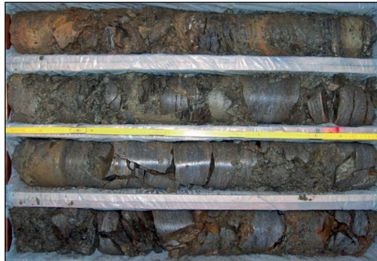
Figure 3.7 Drill core photo, example of cohesive fault rock depicting blocks of various dimensions (cataclasite), after Fasching and Vanek (2011).
